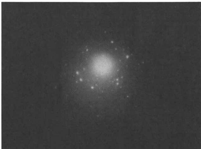
Figure 1. Electron Diffraction Pattern for Cobalt loaded (1 weight %) NaX Zeolite.
